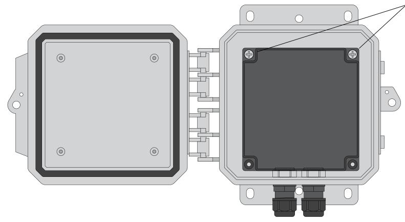
Two Holes for Mounting. Use either top two holes or bottom two holes to mount the receiver.
