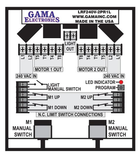
NOTE: The unit is shipped with the limit switches bypassed. To use the limit switches, remove the wire between the limit switch terminals and connect normally closed limit switches as shown.
