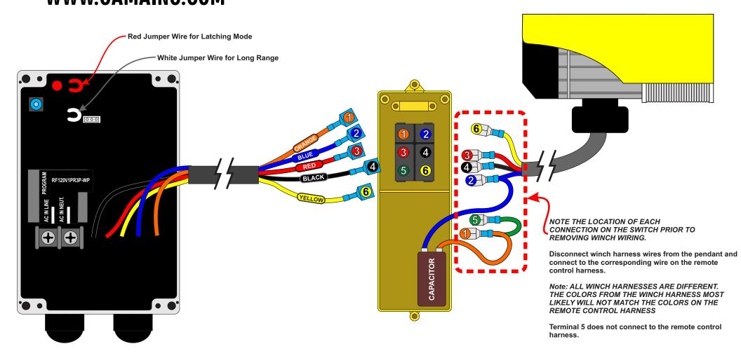
RF120V-1PR3P-WP Pendant Wiring for Winches with Capacitor in Pendant
