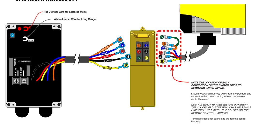
RF120V-1PR3P-WP Pendant Wiring for Winches without Capacitor in Pendant
