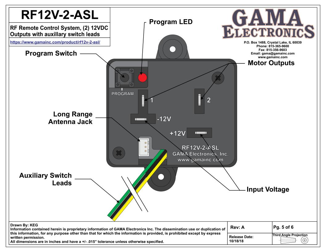
RF Remote Control System, (2) 12VDC Outputs with auxillary switch leads
